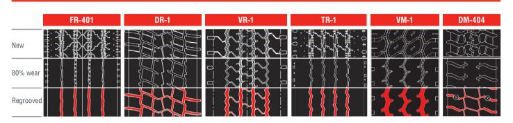
Cost-effectiveness and reliability are the main concerns for professional carriers. "Regrooving" the truck tyres is a Traffic Code approved procedure which allows improving the tyre life.
